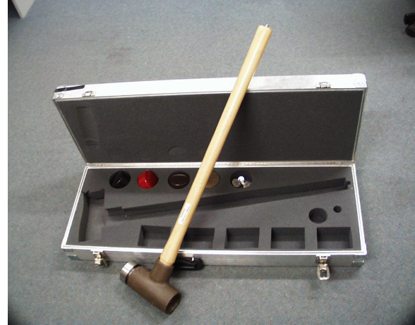
Figure 3 Modally Tuned ICP Sledge Hammer used for bridge tests
