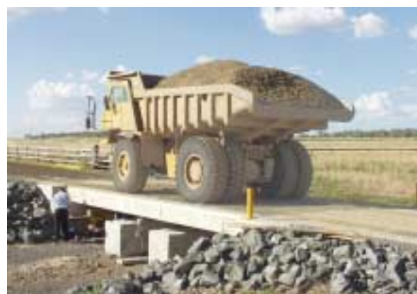
Figure 7 Extreme loading: 75 tonne mining truck with over 45 tonne on rear axle.
