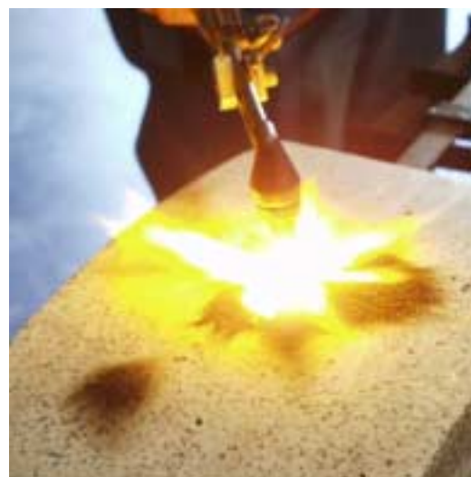
Figure 10 BCC waler under burn test.
