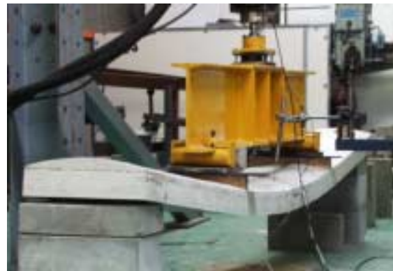
Figure 9 BCC waler under transverse flexural test.
