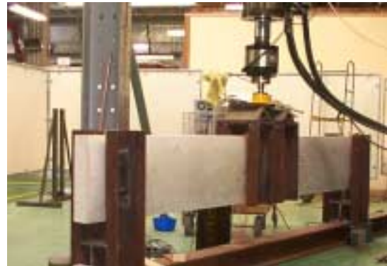
Figure 8 BCC waler under primary flexural test.
