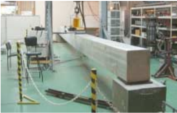
Figure 4 Laboratory testing of 10m beam
