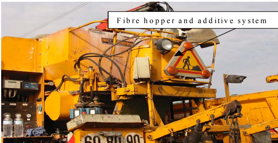
Image 010 – Fibre hopper mounted at rear of slurry machine
