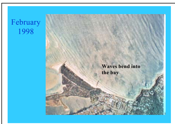
Figure 3 - Wave Crests are misaligned with the shoreline resulting in prevailing longshore currents to the west
